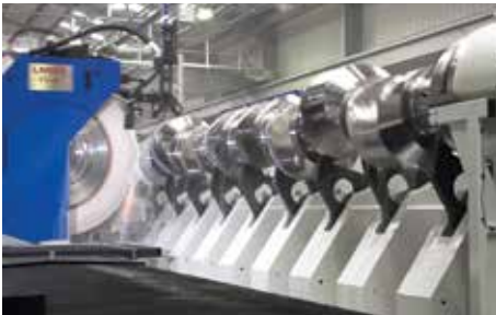
Grinding of pins on 6500mm crankshaft
